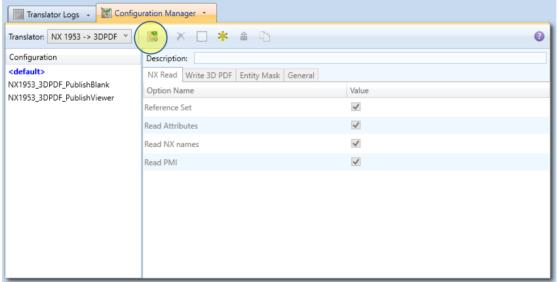
The Configuration Pane allows new configurations to be created based upon ALL available arguments within the Publish 3D application. Selecting the New Configuration icon will allow the user to change any Publish 3D argument.
